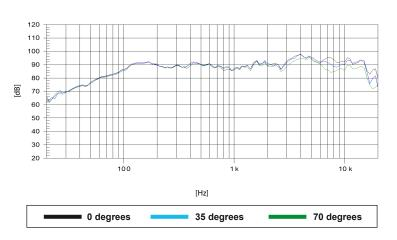
Note: Filtered frequency response measured with loudspeaker standing on infinite baffle in anechoic chamber, 1W @ 1m using filter FD-2CXFe
